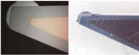
Example of how Koki's 72M solder wire creates a protective barrier on the solder iron tip, extending its life for much longer
