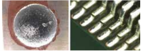
Examples of superior wetting found by using Koki M500C-7 solder paste
